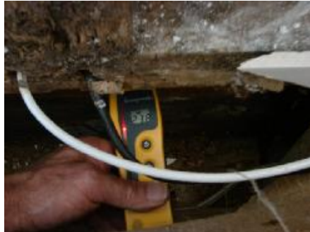
wet boards from hole drill in exterior wall
